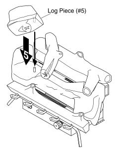
Figure 26 - Installing Log Piece (#5)
